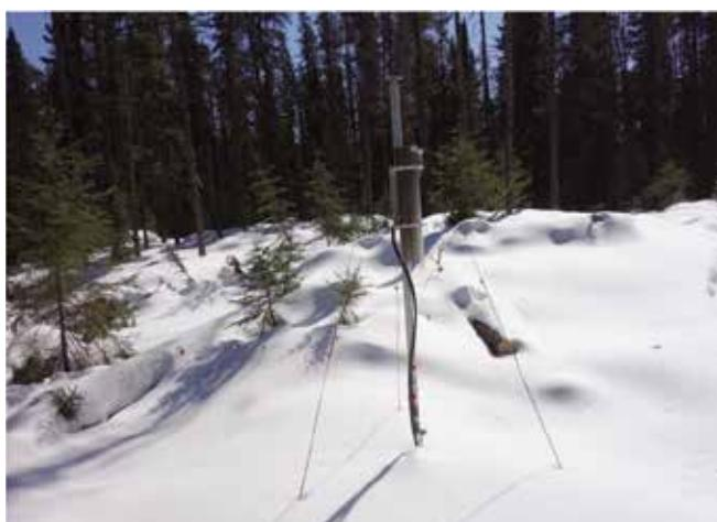
*Figure 2: The GMON snow water equivalent sensor installed at station Mistassibi 2 (Photo by Qing Xiao Zhou)*
